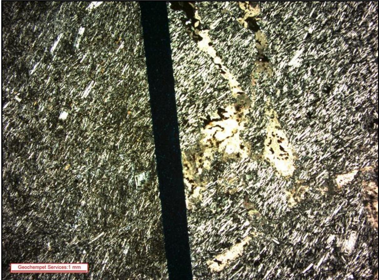
**Plate 2:** Micrograph taken at low magnification, cross polarised transmitted light image of part of trachyte which shows flow-aligned groundmass of feldspar laths with a partly connected network of smectite clay. It shows unaltered feldspar phenocrysts in the left fragment which are completely altered to calcite in the right fragment.
